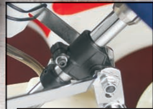
ARROW'S UNIQUE STEERING BUSH WITH CLAMP FOR SIMPLE FRONT END ALIGNMENT
